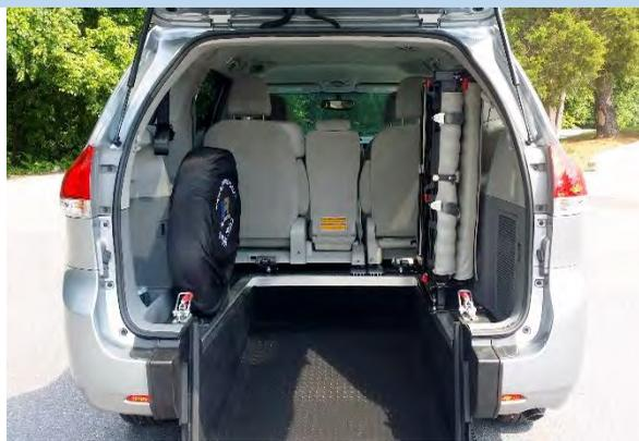
The powder coated, texturized ramp surface reduces slips and improves traction.
